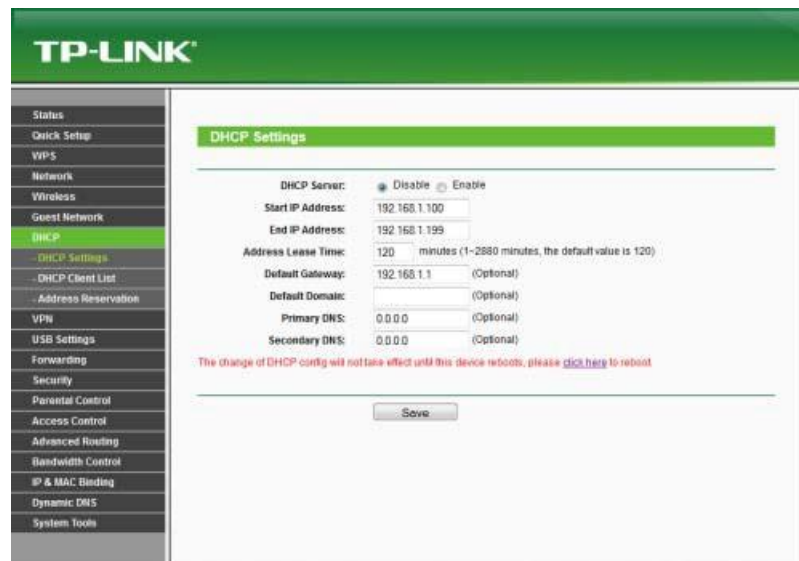
Gambar 4.8 Setting DHCP router 2
